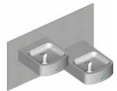
A152400B-FG-W36 Barrier Free, 14 Gage Stainless Steel, Bi-Level, Wall Mounted Drinking Fountain
